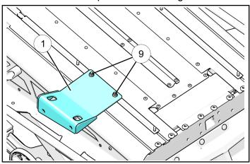
Reinstall the rack support removed in step 4 of the component removal section and torque all six mounting nuts to specification provided.
