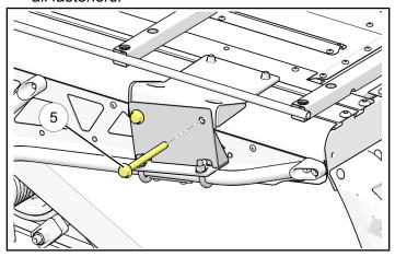
7. Torque the two T-slot nuts (9) previously installed in step 3 of the installation section to the provided specification.
