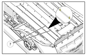
2. Reinstall template making sure tabs are into the opening in the T-slot and newly place bolts are aligned with the holes in the template.
