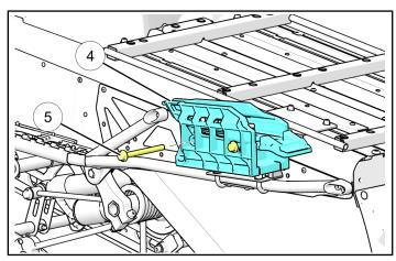
10. Reinstall the rear cargo platform © to the rear rack support using the ten existing fasteners ® previously removed and torque to provided specification.
