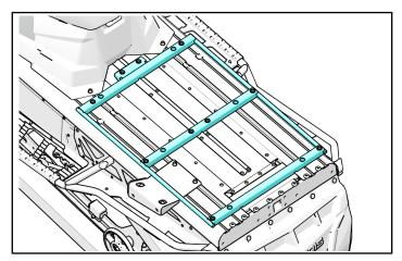
5. Install the mounting bracket as shown using the supplied U-bolts ⑥, nuts ⑧ and washers ⑪. Do not tighten nuts in this step..
