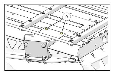
8. Tighten the four U-bolt nuts ®.
