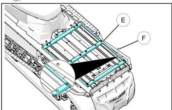
5. Your vehicle is equipped with an aluminum template ⑥ that has pre-drilled holes in it that will need to be removed.
