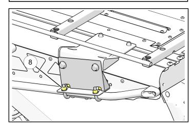
9. Remove the alignment bolts, if not already done, and install the Stronghold Autolatch ④ as shown and fasten into place using supplied bolts ⑤ and nuts ⑩.
