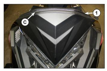
4. Align tabs on bag with the mounting holes in the windshield and windshield trim. Install windshield fasteners (A) through windshield trim, windshield, tabs on bag and through the mounting holes in the hood. Push locking pins into windshield fasteners to lock in place as shown in figure.
