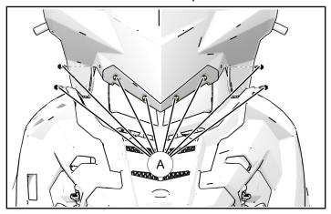
2. Remove the windshield trim®, windshield © and the hood storage bin cover D. The windshield and storage bin cover will not be needed while the Windshield Replacement Bag Kit is installed.
