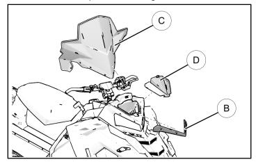
3. Place the Windshield Replacement Bag ① into position and secure by reinstalling the windshield trim ® and securing in place with four push pin rivets A.
