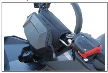
2. Secure hook and loop fastener panels back into place from the rear towards the front of the vehicle as shown.
