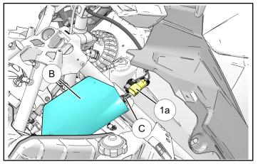
Open bag and connect USB harness connection (1A) to chassis harness connector © as shown.
