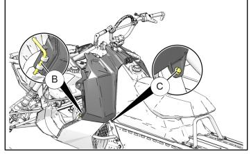
The console should now be in a position to allow you to access the fabric electrical connections bag in the following steps.
