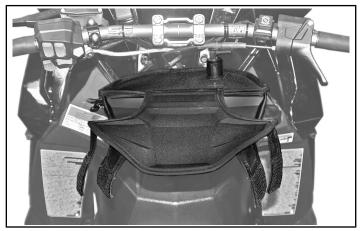
b. Place bag over top of handlebars being sure wires are routed downward along the handlebar post.
