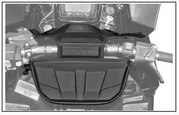
c. Secure bag onto handlebars with the two hook and loop fastener panels on each side of bag.
