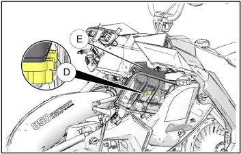
c. Remove the two screws 𝔅 that attach the upper intake plenum 𝔅 to the over-structure along with the two dart clips 𝔅 as shown. Once complete, remove upper intake plenum 𝔅.
