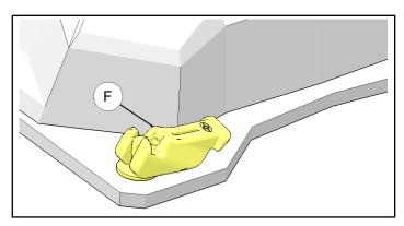
2. Place tunnel bag 1 onto tunnel and place T-slot anchor base into tunnel slot.
