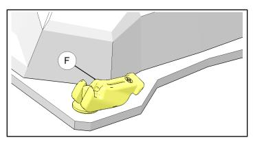
2. Place tunnel bag ① onto tunnel and place T-slot anchor base into tunnel slot.
