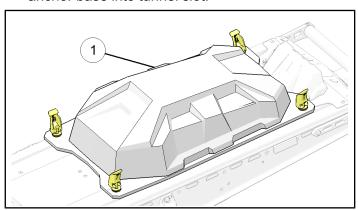
3. Rotate Lock and Ride handle (F) so that T-slot anchor is perpendicular to tunnel slot.
