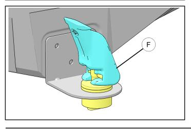
2. Place storage bag ① onto tunnel and place T-slot anchor base into tunnel slot.
