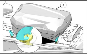
3. Rotate LOCK & RIDE<sup>®</sup> handle (F) so that T-slot anchor is perpendicular to tunnel slot.
