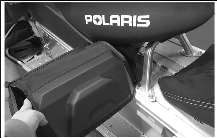
3. Reach inside the bag and push the compression molded panel inside the seat hoop as shown.
