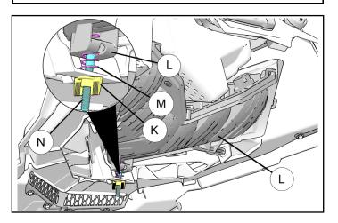
8. Carefully push headlight (L) to the side while gently pushing on the opposite pivot tab (P) enough to release headlight from pivot tab (P) as shown. Disconnect headlight electrical connector and remove headlight from the hood.
