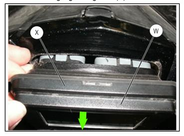
12. Install front and middle hood screens ① ② and upper vent ③ into the hood openings. Using a 3/8" deep well socket gently tap retainers ⑧ onto round tabs in hood to secure screens and upper vent in place.
