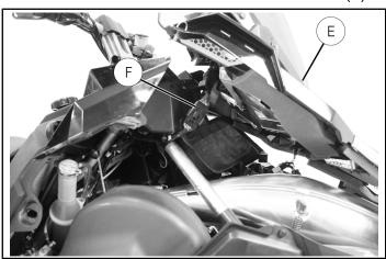
5. Remove hood assembly (E) from the vehicle.
