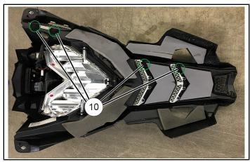
14. Reinstall the gauge into the hood ④. If your sled is equipped with PIDD gauge, install GPS antenna mounting bracket (U) using two screws (T). Install PIDD gauge/sensor onto the mounting bracket (U).
