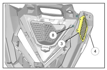
13. Install six foam insulation pieces and 4 fabric patches from the foam kit (10) in the locations as shown on the hood (4).
