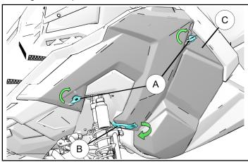
2. Open the side panel (C), then pull the panel outward to release the tabs at the bottom. Repeat the same for removing side panel on other side of vehicle.
