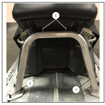
6. Place new seat support onto carriage bolts ②. Install nuts ③ and washers ④ from top to secure seat support.
