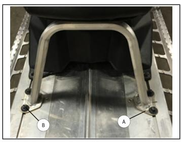
2. Remove two M6 X 1.0 mm nuts (B) from seat base bolts (C).
