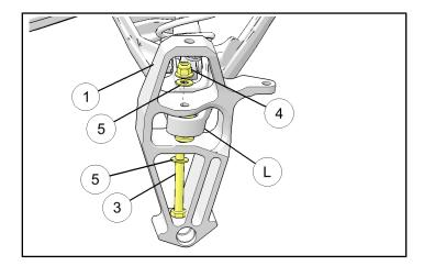
8. Place upper control arm (K) onto spindle ①. Ensure washers ⑤ are placed on top and bottom of spindle and tighten using 8 mm Allen wrench and 15 mm wrench. Torque to specification.
