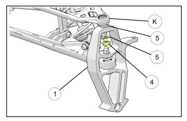
9. Place tie rod (H) onto spindle ①. Make sure to place washers ⑥ on top and bottom before tightening tie rod using 13 mm and 17 mm wrenches. Torque to specification.
