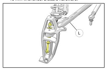
7. Place new spindle ① onto lower control arm (L), install M10 screws ③ from bottom up, ensure washers ⑤ are properly in place and securely fasten using two 15 mm wrenches. Torque to specification.
