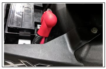
10. Install red positive (+) battery harness cable along with all other required red positive (+) cables with new longer battery bolt and threaded battery post block that was provided with your kit to the positive (+) battery terminal. Then install the black negative (-) battery harness cable and all other required black negative (-) cables to the negative (-) battery post with new provided battery connection hardware.
