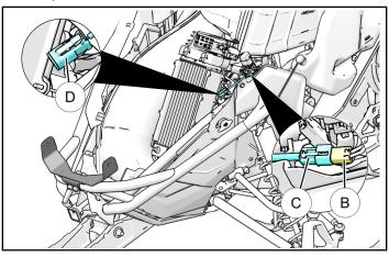
b. Route the remaining portion of the harness forward along the top of the inner bumper tube to be connected to your specific accessory light's electrical harness.
