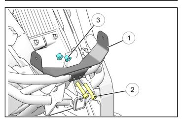
c. After torquing the bolts, install the two provided locking nuts ③ onto bolts ②. To do so, hold the bolts firmly in position and torque the locking nuts to specification provided. Ensure that the bolts do not turn while torquing the locking nuts.
