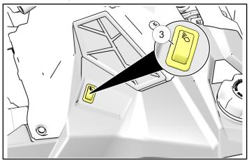
f. Connect switch to existing electrical connector
