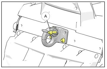
2. Install the Titan 1.25" Receiver onto the rear of the snowmobile as shown using the supplied four new bolts ④. Torque to specification.
