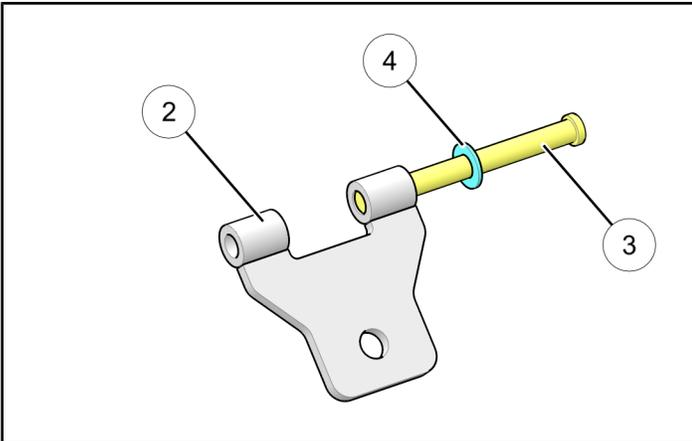
2. Place hitch mount ① into position as shown and fully insert the hitch pin ③.
