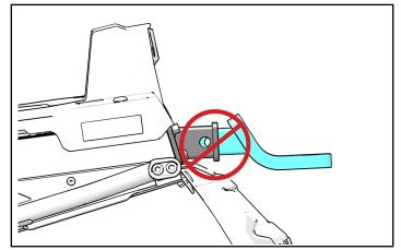
3. Fully insert the hitch pin and secure in place using the cotter pin that was provided with your Titan Ball Hitch Receiver Kit (PN 2882795).
