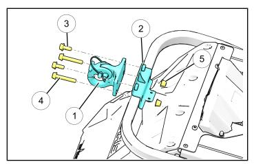
3. Using a pop rivet puller and the provided rivets ① and washers ⑥, rivet the hitch adapter to the snow flap.
