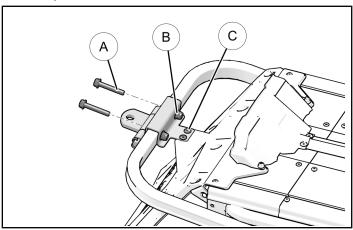
Using the provided screws 3/4 and locking nuts
