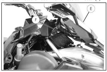
6. Remove the hood assembly (E) from the vehicle.
