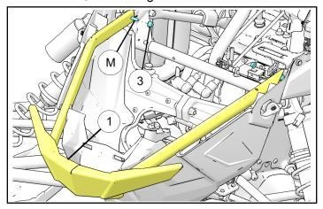
2. Install two Torx® screws ② and secure left and right side of bumper ① to the nose pan.
