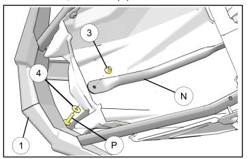
4. Tighten all fasteners to specification at this time.
