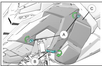
Open the side panel (C), then pull the panel outward to release the tabs at the bottom.
