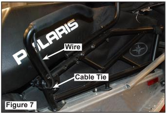
24. Connect RH and LH hand warmers to accessory hand warmer harness. Make sure hand warmer harness has one to two inches of slack between fuel tank and rack. Figure 8. Wire should be run on the front side of rack tube. Bundle together any unused length of wire harness and tape to rack with electrical tape. Secure wiring 3" from inside tube of rack with cable ties. Figures 9 and 10.
