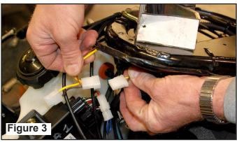
12. Loop harness that goes to switch over top of steering hoop left of steering post. Figure 2. Secure hand warmer harness to main harness with cable ties as shown in Figure 4.
