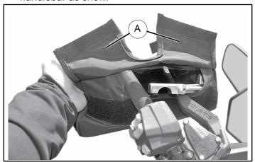
2. Pull gauntlet completely over handlebar controls and into position as shown.
