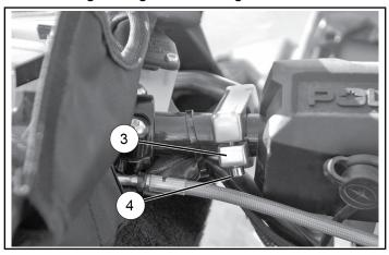
4. Torque mounting screws ④ to specification listed below.
