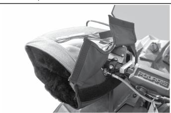
3. Place the lower mounting clamp 3 into position as shown and loosely start the two mounting screws4) by hand until they are slightly snug.
