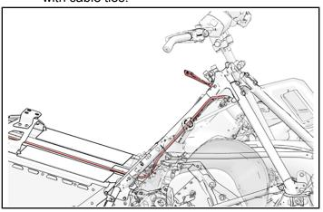
The heated grip connection should end up in the approximate position shown below.
