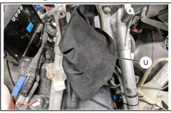
Connect the white 12V power connector to the matching RCA accessory power connector on the main harness as shown and replace protective cover.
