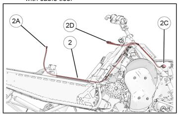
Start by placing fuse holder in the approximate position shown below. Secure into position with a cable tie.
