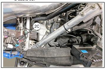
Continue upward along the front left hand overstructure tube routing the harness underneath the steering support structure so the white 12V power connector is in the approximate location shown. Secure to support tube with cable ties.
