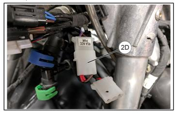
Route remaining harness over to and down the rear right hand over-structure tube along side the tail light harness wire. Continue along the top surface of the tunnel along side the tail light harness as shown below. Secure into position with cable ties.
