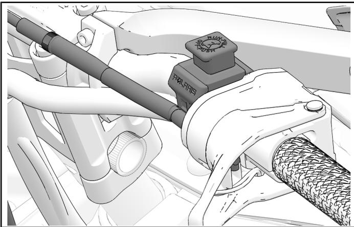
8. Once in the proper position, torque mounting fasteners ⑩ to specification.
