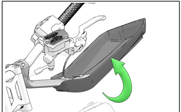
3. Verify that the handguard assembly does not interfere with the brake mechanism. Make sure that the parking brake locking mechanism is free to rotate into the fully locked position and does not make contact with the upper mount or any other portion of the handguard assembly.
