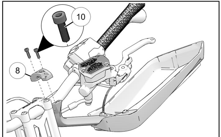
2. Carefully rotate the handguard assembly upward and into position.
