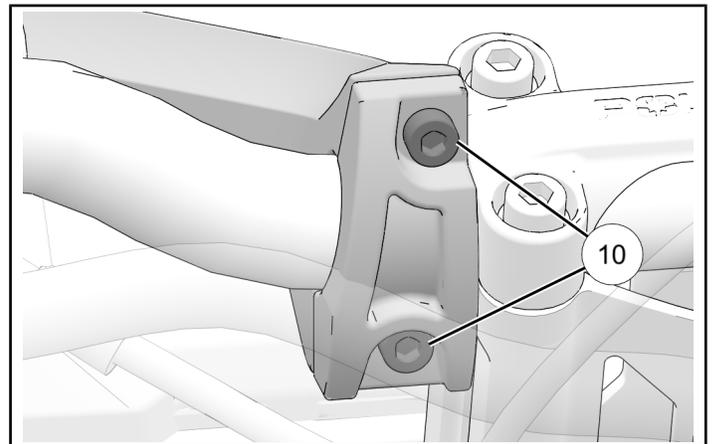
5. Place RH handguard assembly into position as shown. Loosely install the RH mounting cap ⑥ using supplied fasteners ⑩.
