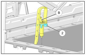
To secure accessory: Wrap strap ③ through accessory ring or handle, then wrap strap back to bracket ③ and secure to tab. Ensure tab on bracket fully engages hole in strap. Repeat for opposite side.
