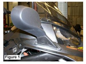
Install the mirrors and secure with screws and nuts supplied with the kit. Torque to 6-8 in. lbs. (0.68-0.90 Nm) Figure 2.
