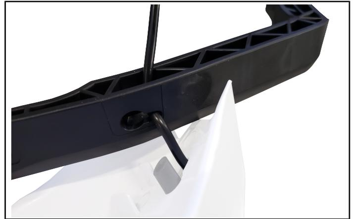
18. Move the RH lighted cap wire harness into the wire harness slot and carefully install the RH lighted cap onto the handguard.
