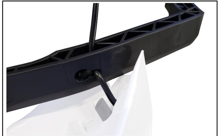
12. Carefully install the LH lighted cap / handguard onto the mount and make sure the wire is not pinched between the mount and handguard.
