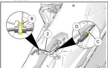
b. Connect the black plastic lower jumper harness connector ① to the existing connector © on the chassis harness as shown.
