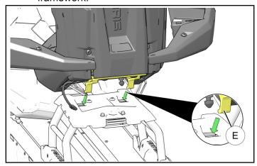
b. Once the seat support hooks are fully engaged, press down firmly on the rear of the seat so that the seat latch pin (£) engages the latching mechanism.
