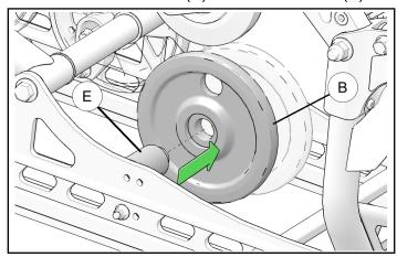
Repeat Step 2 and Step 3 for other side wheel removal. 5. Mount new bogie wheel ① on wheel mount (E).
