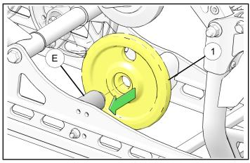
6. Install screw ② with washer ④ and nut ③ on new wheel. Note bolt and washer orientation. Torque nut ③ to specification.
