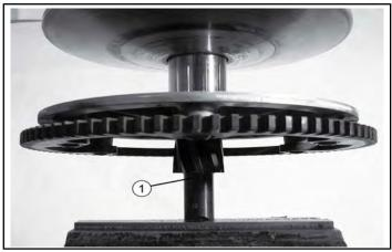
b. Check crankshaft taper for galling or scoring. If necessary clean the taper evenly with 200 grit emery cloth.
