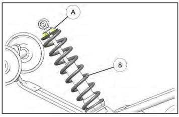
d. Reinstall upper shock mounting bolt ® and nutA. Torque to specification.
