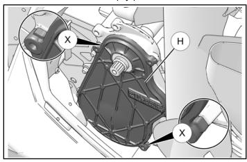
e. After removing the cover, note the two dowels in the chaincase.
