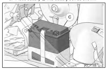
b. First connect the red positive (+) solenoid cable to the positive (+) battery terminal using the battery cable connection hardware supplied with your battery. Torque battery connection hardware to specification provided.
