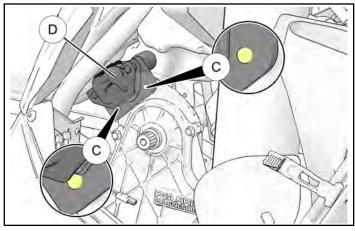
c. Torque fasteners © to specification.
