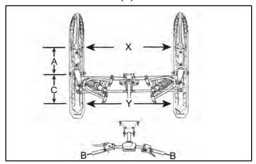
11. Once the proper measurement is obtained ensure the tie rod ends have equal thread engagement. Both inner and outer rod ends should also be parallel to allow the steering to be turned fully in both directions with no binding on the tie rod ends. Once you have verified there is no binding and there is equal thread engagement torque both inner and outer jam nuts on each tie rod to specification.
