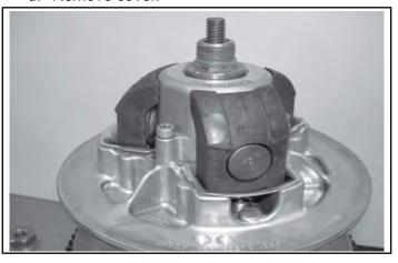
e. Remove the three sliding blocks ① from the sheave.
