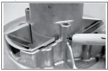
i. Remove the screws © securing the cover to the moveable sheave. Slowly release the clutch compressor and remove the spring cover.
