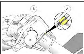
Reconnect throttle cable. Be sure cable is fully seated into new throttle flipper.
