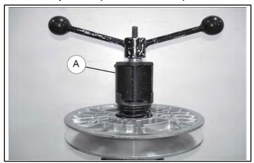
b. Compress driven spring enough to access and remove the snap ring.
