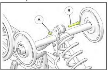
b. Using a spring compression tool, compress spring and remove spring retaining collar (A). Remove spring compression tool and then remove spring (B).
