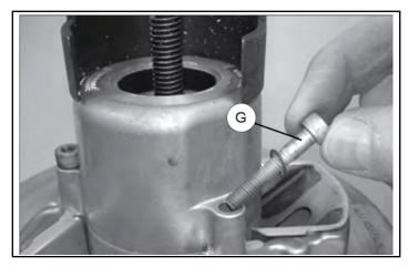
c. After tightening spring cover screws, slowly remove the clutch compressor (£) from the spring cover (£).
