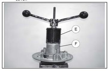
h. Mark the cover and moveable sheave with a permanent marker.
