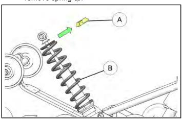
c. Install provided spring (a). Using the spring compression tool, compress the spring and reinstall the spring retaining collar (a). Then remove spring retaining tool.
