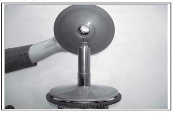
h. Install the sliding blocks ① into the moveable sheave. Verify the curved sides are upwards and the straight sides are down.
