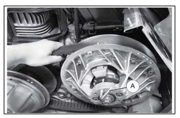
b. When the clutch sheaves are opened, remove the drive belt from the driven and then drive clutch.
