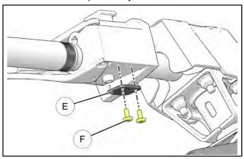
e. Install throttle pin ® and secure with E-clip ® being sure the supplied spacers are installed in the original locations to allow free movement of the throttle flipper.
