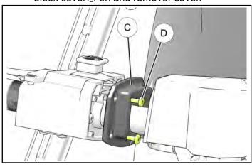
d. Remove the two screws and wire retaining cover to allow the heated throttle flipper wire and throttle flipper to be removed.
