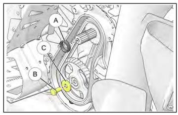
c. Rotate the driven clutch forward to move all of the chain slack to the tensioner side.
