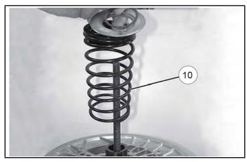
b. Compress the spring stack into the clutch using the Universal Spring Compressor. Compress stack enough to expose the snap ring groove in the fixed sheave shaft.
