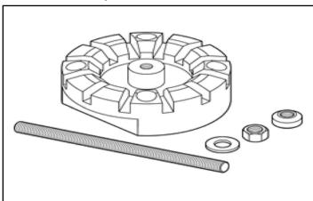
b. Place the drive clutch assembly onto the fixture tool and secure to base. Remove the nut (A) and flat washer (B) from the clutch assembly.
