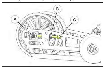
c. Once the adjuster bolts are fully retracted, push the rear idler assembly ① forward.
