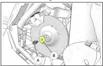
b. Release the parking brake. Remove the brake caliper mounting bolts ©. Tie the caliper D to overstructure.
