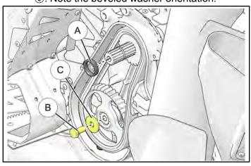
c. Loosen the chain adjuster screw and remove the tensioner pad.
