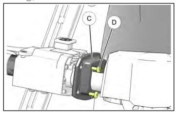
d. Reinstall the wire retaining cover (£) and secure with the two previously removed screws (£).
