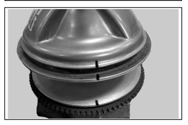
a. Place the **Drive Clutch Holding Fixture (PN: 2871358-1)** in a bench vise.
