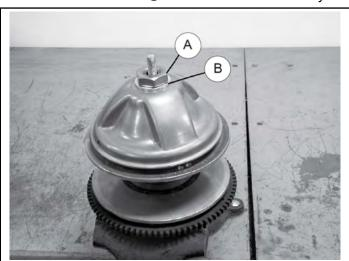
c. Mark © the stationary shaft and cover with a permanent marker as shown .
