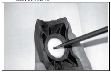
b. Remove the shims (A) from the blocks.
