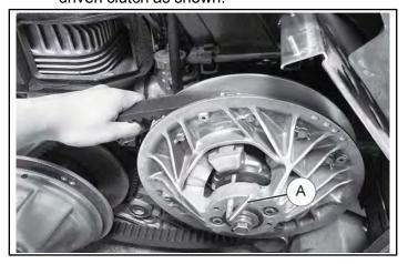
c. Remove the L-Wrench tool and work the belt to the top of the sheaves on the driven clutch.
