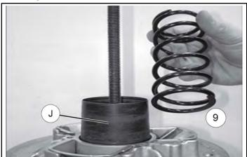
b. Install the spring cover making sure the alignment marks between the cover and moveable sheave made during disassembly are aligned. Slowly compress the spring cover down using the Universal Clutch Compressor. Reinstall the screws © and torque to specification.
