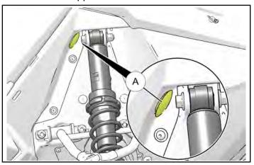
c. Remove upper locking nut ® and slide upper bolt A out through the access hole in the fender while firmly holding shock.
