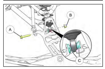
b. Next, remove the rubber plug (A) in the fender to allow upper shock bolt removal.
