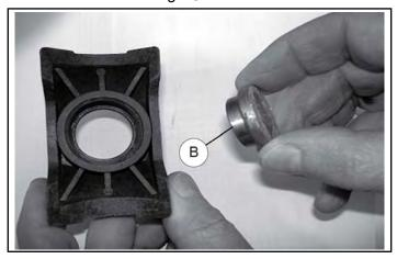
d. Install the new provided slugs ③ into each sliding block in the same orientation as the original.
