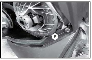
c. Slide the driven clutch off of the jackshaft.
