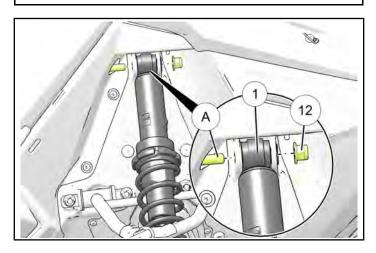
b. Place lower end of shock into position using previously removed spacers (a) and bolt (a). Secure with provided locking nut (1) and torque to specification.
