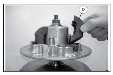
f. Remove moveable sheave and place into the Universal Clutch Compressor, PN: PU-50518–A g. Tighten clutch compressor against spring cover.
