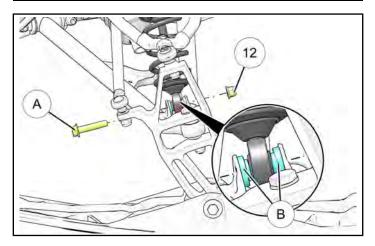
c. Reinstall rubber plug (A) into fender.
