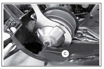
d. Tighten the puller into the clutch. If the clutch does not come off, strike the clutch puller head with a hammer. If the clutch does not "pop" off, continue to tighten the clutch puller, and repeat this step.
