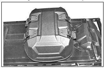
Check that the bag is secure by gently pulling up on each corner of the bag to ensure all Lock & Ride anchors have been fully engaged in the Tslots on the tunnel top.
