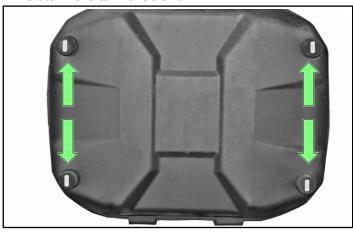
Once aligned, place bag onto tunnel being sure all four anchors are fully seated into the T-slots and slide the bag into the desired position.
