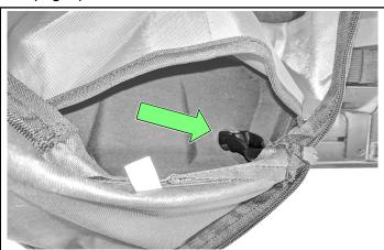
Next, rotate the Lock & Ride anchors so the lower portion of all four anchors are parallel with the Tslots in the tunnel as shown.
