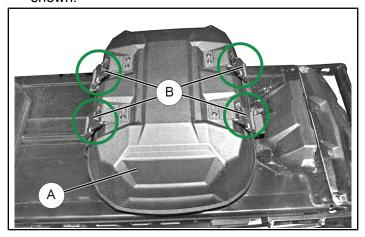
3. Unzip bag to gain access to Lock & Ride anchors. Make sure the Lock & Ride anchors are in the upright position as shown.
