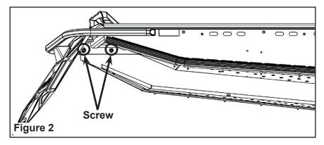
3. Install the trailer receiver hitch (1019585) with four cap screws and nuts. There are two sets on each side. Figure 3.
