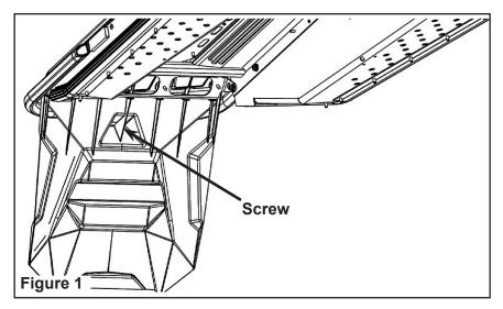
2. Remove the four Torx T27 screws connecting the bumper to the frame. There are two screws on each side. Figure 2.
