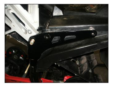
3. Drill out the rivet (C) that fastens the snow flap to the bumper. Remove the bumper from the vehicle as shown in figure.
