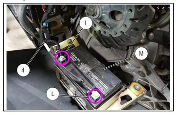
10. Install Panduit strap with Christmas tree clip (8) onto the harness (4) at the white tape closest to terminal and install clip into hole on the tab of the battery box as shown.
