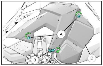
2. Open the side panel (C), then pull the panel outward to release the tabs at the bottom. Similarly, remove side panel on other side of the vehicle.
