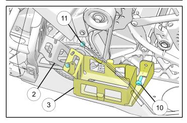
For Trail Performance Models: Insert two studs on stud plate ① through holes on RH footrest (K) from underside as shown. Hold stud plate in this location and mount the battery box ③ onto studs and install two nuts ①. Mount the battery box to bulkhead side using one screw ⑩ as shown. Use 10mm wrench for nuts ① and T40 Torx<sup>®</sup> for screw ⑩ installation.
