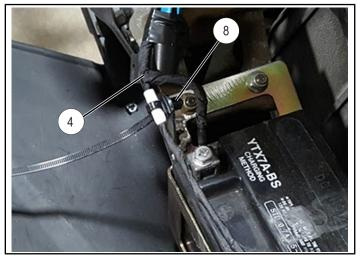
11. Install harness mounted Christmas tree clip (P) to the white tape nearest to main harness plug and install onto the hole on the aluminum tube as shown.
