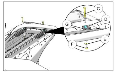
4. Generously lubricate full length of inner channel on wear strips ① with a strong soap and water solution. Starting from under the tunnel close off, with the holes in wear strips towards the rear, start wear strips onto the mounting extrusions ④ on the underside of the tunnel. Slide the wear strips on full length of tunnel mounting extrusions stopping when holes in wear strips line up with holes in tunnel from original track protector strips.
