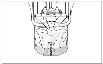
Complete snow flap installation by reinstalling the previously removed snow flap fastener (A) and plate (B) to the underside of the snow flap and into the rear bumper as shown.
