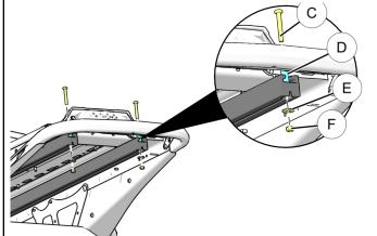
6. Reinstall snow flap using the provided four rivets②.
