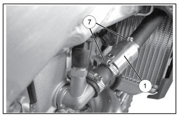
g. Reinstall pressure line onto vehicle being sure to secure with previously removed hardware.
