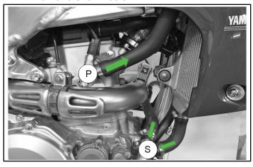
b. Place the thermostat next to the pressure line to determine where it would fit best.
