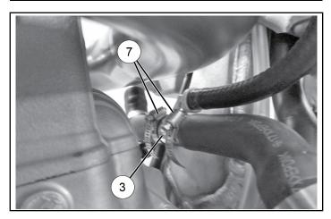
Reinstall hose back onto vehicle being sure to secure hose with previously removed hardware.
