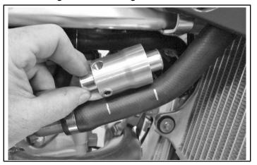
d. Remove pressure line and cut on your marks.
