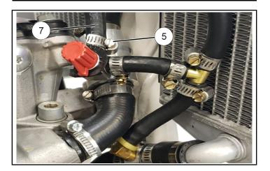
e. Once you have verified hose length and that there is no interference with the steering components, cut the hose to length and install the provided flared push lock fitting on the open end of hose as shown. A hose clamp is not required on this fitting.
