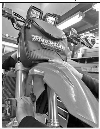
5. Mount the upper TRIO mounting bracket as shown to the top of your TRIO shock using the supplied bolt. Make sure the Upper TRIO bracket is facing forward in relation to the bike and the TRIO shock reservoir is positioned towards the rear of the bike. Torque to the specification listed below.
