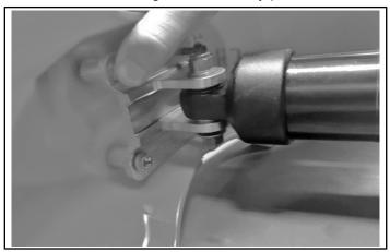
8. Remount fender and TRIO assembly to the underside of the motorcycle's lower triple clamp. Torque to the specification listed below.
