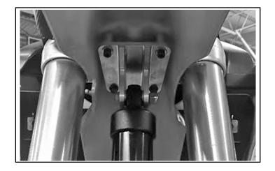
9. Place the lower eyelet of the TRIO shock into the original rear spindle block spacer location. The Timbersled TRIO shock is designed to have around ¼" of pre-load when installed. This may cause the TRIO shock to appear to be too long when mounting into the rear spindle block spacer location.
