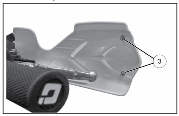
6. Place Hand Gauntlet over the front of the hand guard snapping the outer snaps © to the newly installed mounting snaps on the front side of the hand guard.
