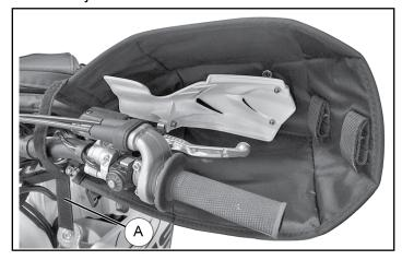
3. Once Hand Gauntlets are in desired location use a pencil or marker to mark the center of each mounting snap location (B) on existing hand guard shield.
