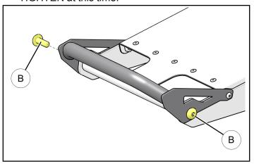
5. After starting all mounting bolts by hand, torque the forward most bolts ② to specification provided starting with the left side (drive-side) bolt FIRST followed by the right side.
