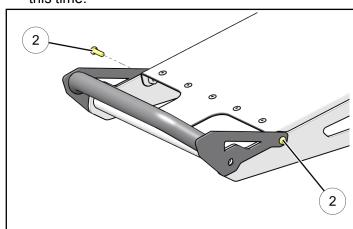
4. Next apply LOCTITE® 243™ Blue to the two rear most bolts ® previously removed and reinstall into two rear most mounting holes as shown. DO NOT TIGHTEN at this time.
