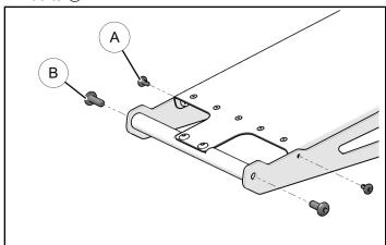
Place ARO Extreme Bumper ① over the top and outsides of the tunnel as shown being sure to line up the mounting holes with the side panel bolt holes.
