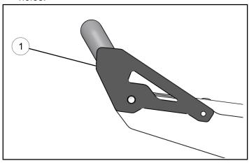
3. Apply LOCTITE® 243™ Blue to threads of provided two bolts ② and install into the forward most mounting holes as shown. DO NOT TIGHTEN at this time.
