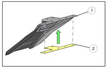
b. Next place snow flap/reinforcement plate assembly ①/② into position on the underside of tunnel as shown, using supplied rivets ③ to align into proper position.
