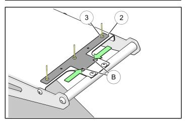
b. Once the plate is temporarily secured into position use a drill and 3/16" (5mm) drill bit to drill new holes (a). After drilling, clean all shavings left from the drilling process from the top of the tunnel and remove plate.
