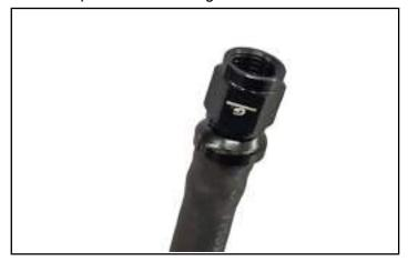
After installing fitting, connect hose to mating fitting on left hand side of handlebar. This threaded connection DOES NOT require thread sealer.
