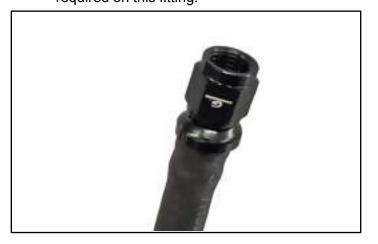
f. After installing fitting, connect hose to mating fitting on right hand side of handlebar. This threaded connection DOES NOT require thread sealer.
