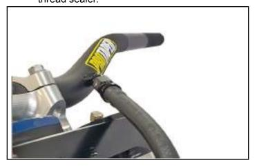
d. Next, attach the remaining hose to the upper leg of the control valve, being sure to install provided hose clamp, and route to the right hand handle bar fitting. Ensure handlebars can be turned side to side without causing any interference to the hose. When finished, be sure to tighten hose clamp to specification.
