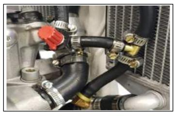
b. Once you have verified hose length and that there is no interference with the steering components, cut the hose to length and install the provided flared push lock fitting on the open end of hose as shown. A hose clamp is not required on this fitting.
