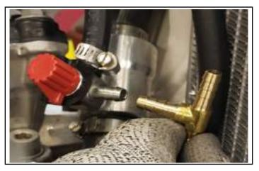
ii. Once located, mark and cut the bypass hose and install the barbed tee fitting. This junction requires a hose clamp so be sure to place a provided hose clamp onto the bypass hose BEFORE pushing hose onto fitting.
