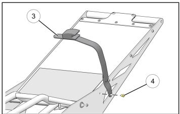
Install ladder strap (2) to non drive side panel in the location indicated below using the supplied fasteners (4) as shown. DO NOT use flat washers on Timbersled RAW kits.
