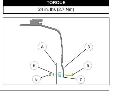
Install ladder strap 2 to non drive side panel 8 in the location of the previously removed screw using the supplied fasteners 5,6,7 and 8 as shown.
