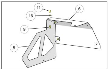
3. Install RH panel ④ onto the underside of the front panel ⑥ by lining up the three bolt holes of each panel and fastening the two panels together using the provided gas rack panel bolts ⑨, washers ⑯ and acorn nuts ⑪ as shown inserting bolts ⑨ from the inside of the rack out. **DO NOT** tighten at this time.
