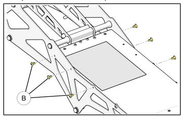
7. Place the loosely assembled fuel can rack over the tunnel lining up the side panel mounting holes as shown. Install the provided side panel bolts ® as shown on each side. **DO NOT** tighten at this time.
