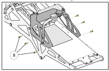
8. Install front and rear cross shafts ③ by inserting inbetween the two fuel can rack side panels and lining up the mounting holes as shown. Fasten using provided gas rod bolts ⑧ and washers ⑩ as shown. **DO NOT** tighten at this time.
