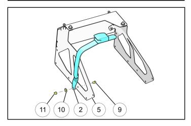
5. Next run the right hand ratchet strap ① on the outside of the RH side panel ④ of the gas rack as shown and fasten to the outside of the panel using provided ratchet strap bolts ⑨, nut ⑪ and washer ⑩. Torque to specification listed below.
