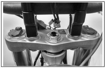
3. Remove rear bolt (A) and aluminum spacer (B) from ski mounting block on spindle.
