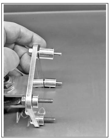
7. Place the fender onto the TRIO shock assembly with mounting bracket and hardware as shown. Ensure that the mounting hardware, upper TRIO bracket, spacers, and fender are lined up and the hardware is through all necessary pieces.
