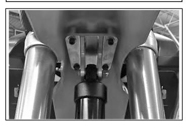
9. Place the lower eyelet of the TRIO shock into the original rear spindle block spacer location. The Timbersled TRIO shock is designed to have around ¼" of pre-load when installed. This may cause the TRIO shock to appear to be too long when mounting into the rear spindle block spacer location.
