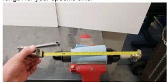
11. The strut rod length for your specific bike is a center to center measurement.
