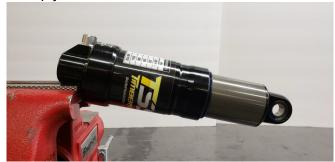
5. Apply a small amount of LOCTITE® Threadlocker Blue 243® (or equivalent) to the shaft ® threads.
