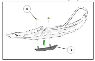
Install new skag ① onto ski with the carbide inserts oriented towards the front of the ski as indicated in the inset ⑥. Secure with provided locking nuts ②. Torque to specification listed below.
