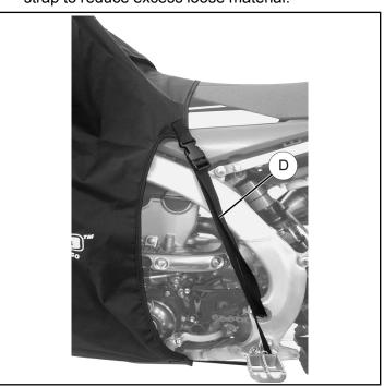
8. Verify that the fuel access port has been zipped closed and readjust all straps as necessary to ensure there is no excess loose fabric.
