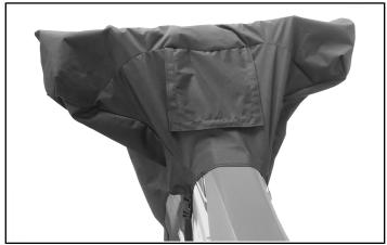
5. Once the cover is fitted to the vehicle, secure the front spindle hook strap (B) to the lower-most edge of the front spindle plate as shown.
