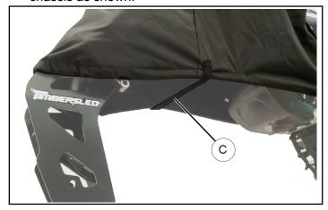
Next, run the lower side tensioning strap back around the foot peg of the snow bike and back up to the female half of the cover's buckle. Tighten strap to reduce excess loose material.
