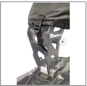
6. Secure the hook and loop cover strap © in between the front forks/spindle and the snow bike chassis as shown.
