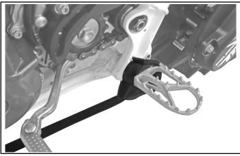
3. Next, connect to towing vehicle by feeding carabiner and strap around rear bumper and clipping the carabiner strap to one of three loop strap locations to achieve the desired tow rope length.
